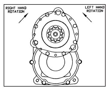
Figure 1. Direction of Rotation viewed from Pinion End.
