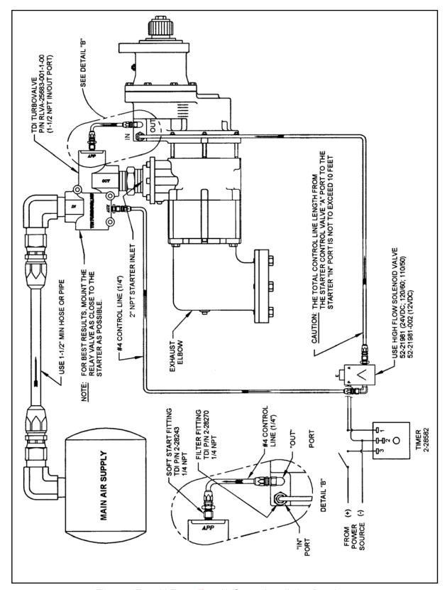
Figure 4. T100-V TURBOTWIN Air Starter Installation Drawing
